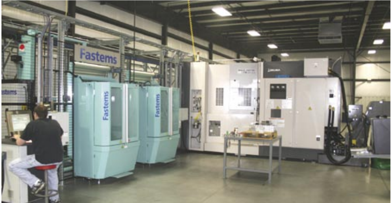
Above: One of C.E. Machine's crew is dwarfed by the new Okuma Fastems FMS horizontal machining cell. Purchased through Hartwig, it features 48 pallets, 50-tool magazine with tool management software and a 12,000-rpm spindle.
